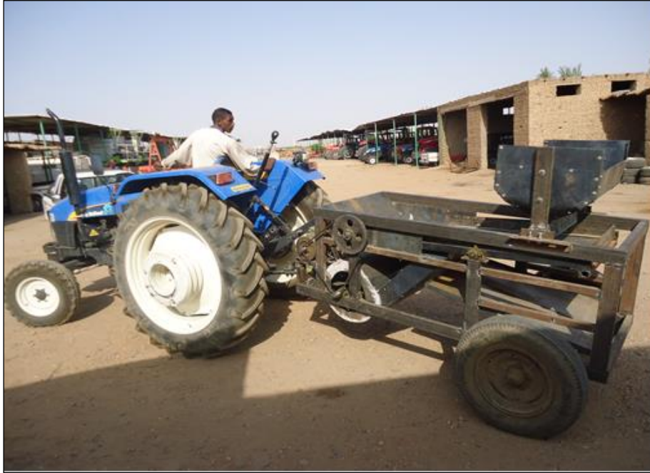
Figure 3: The prototype of wheat cleaner
