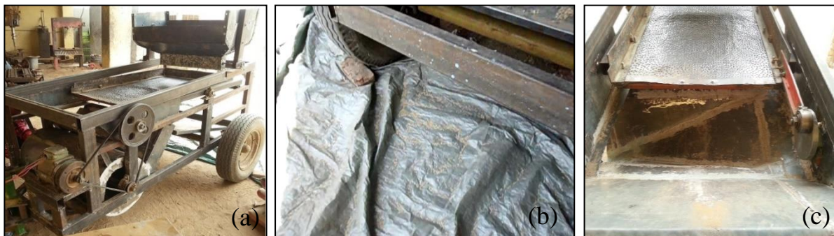
Figure 2: (a) the prototype of wheat cleaner, (b) undesirable materials, (c) clean grain pan
