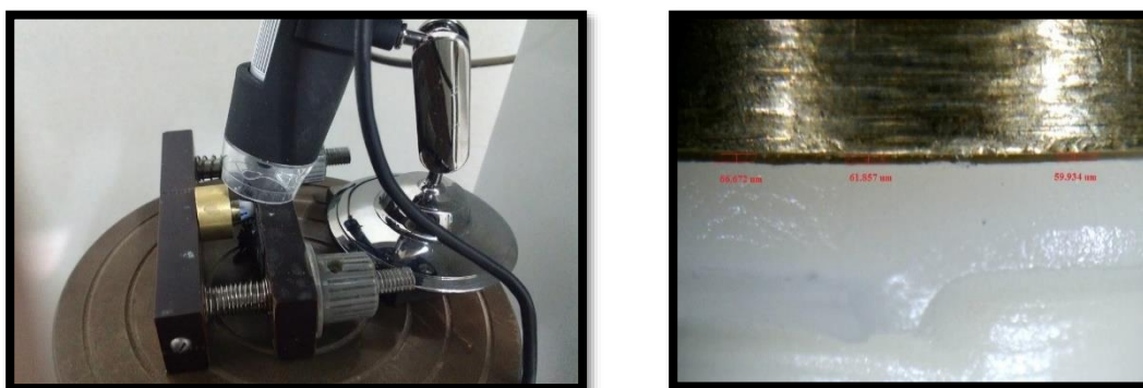
Figure (20 a,b ) Olympus camedia C-5060 digital camera fitted on Carl Zeiss Stereomicroscope
