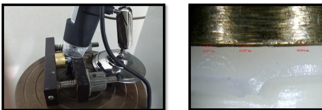
Figure (20 a,b ) Olympus camedia C-5060 digital camera fitted on Carl Zeiss Stereomicroscope
